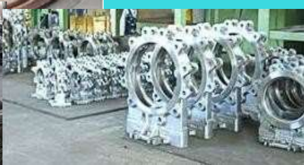
Valve Casting Ready for Machining
