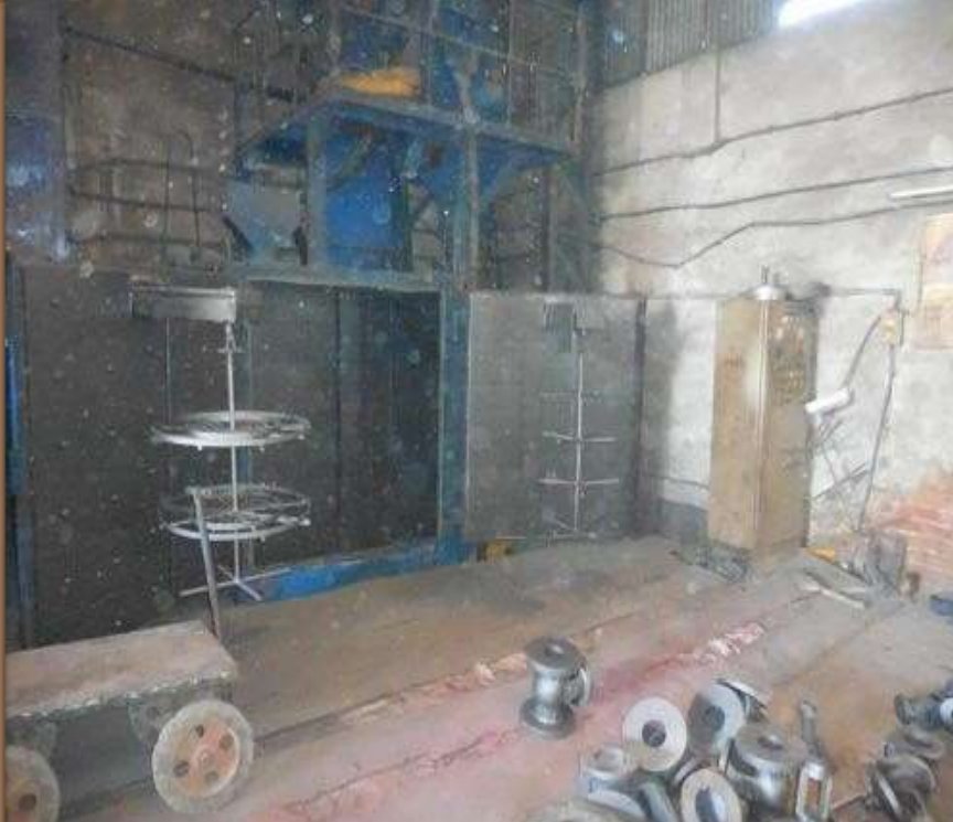
Our Sort Blasting Machine to Clean the Casting.
